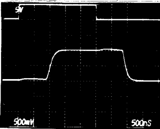
MUX-24 SMALL-SIGNAL SWITCHING WITH FILTERING AND 2.5 \mu s SAMPLE TIME
